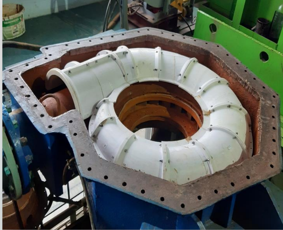
Model block, spiral casing, and runner of a high-speed pump-turbine model
