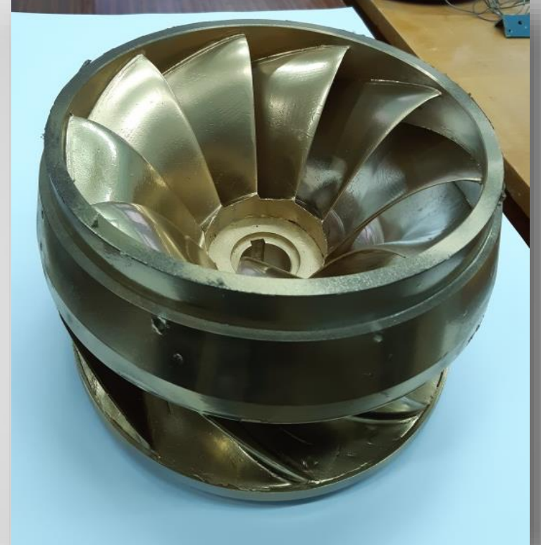
Model block, spiral casing, and runner of a high-speed pump-turbine model
