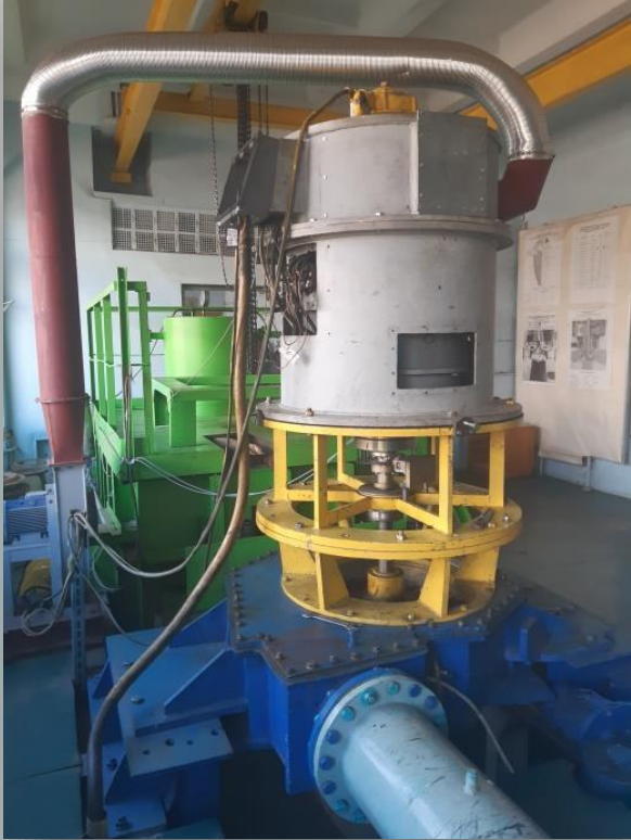
Model block, spiral casing, and runner of a high-speed pump-turbine model
