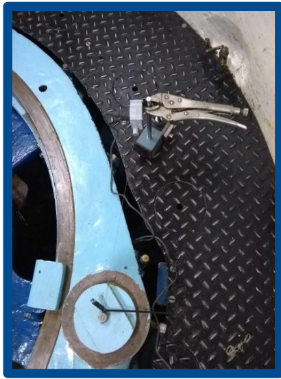
Measuring the movement of the WG ring
